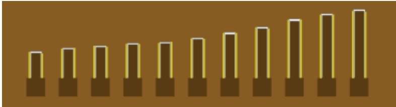
Rotate the reedplate 90 degrees and emboss the tips of each slot.
