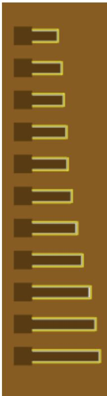
Plink each reed and repeat the centering and deburring process until each reed is free.
