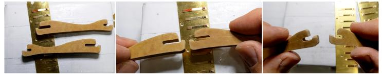
The short end is easier to use. Since the most common defect is a curvature in the middle of the plate, you will be using the short end most of the time.
